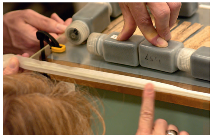
8. Sealing with Filmoplast p-90.
