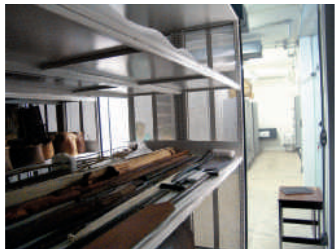
4. Side panels of compact shelving system are made of perforated plate in order to allow air flow through the panel even in closed positions.
