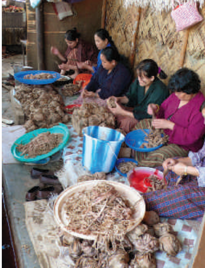
1. Women peeling the bark of wet raw plants. Depending on the quality of the original fiber and the beaten process, at least two different grades of paper are obtained. Jungshi Hand-made Paper Factory, Thimphu. Bhutan.
