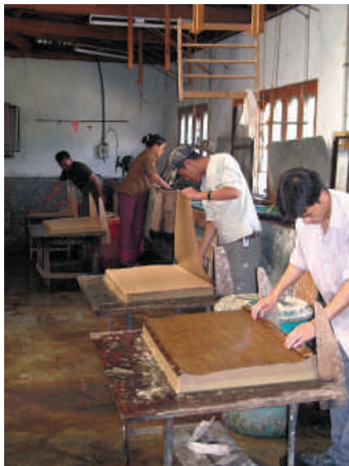
2. Workers placing the sheets of paper freshly made on the stacks of paper using flexible screens made of bamboo. Jungshi Hand-made Paper Factory, Thimphu. Bhutan.
