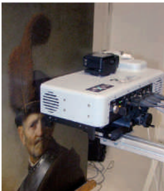
9. The portable XRD/XRF is ready to analyze the pigments of underpainting in the An Old Man in Military Costume by Rembrandt van Rijn, property of the J. Paul Getty Museum. Photo: Giacomo Chiari.
