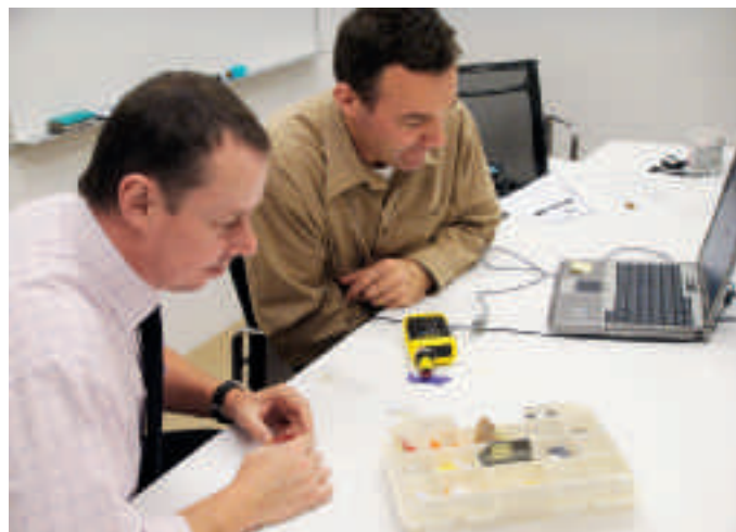
4. GCI scientists Alan Phenix (left) and Tom Learner assessing the potential of a small, handheld Raman instrument for rapidly differentiating classes of plastic. Photo: Rachel Rivenc.
