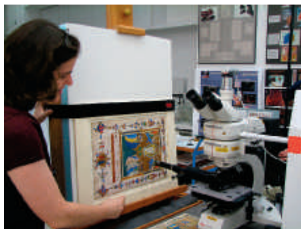
2. An illustration in Martín de Murúa's Historia general del Piru , being examined by GCI scientist Catherine Patterson using Raman spectroscopy. Photo: Dennis Keeley.
