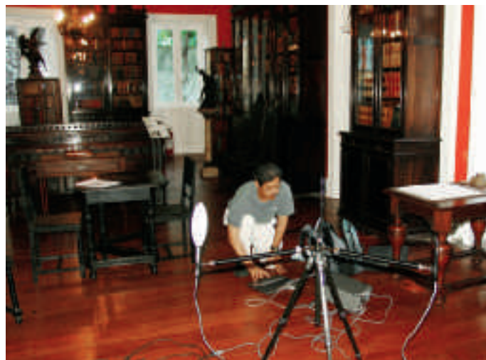
3. GCI scientist Shin Maekawa takes temperature and humidity measurements in the library of Casa de Rui Barbosa. Photo: Claudia Carvalho.
