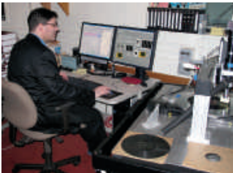
5. LC's IRENE Machine can capture sound using light rather than a stylus. © LOC
