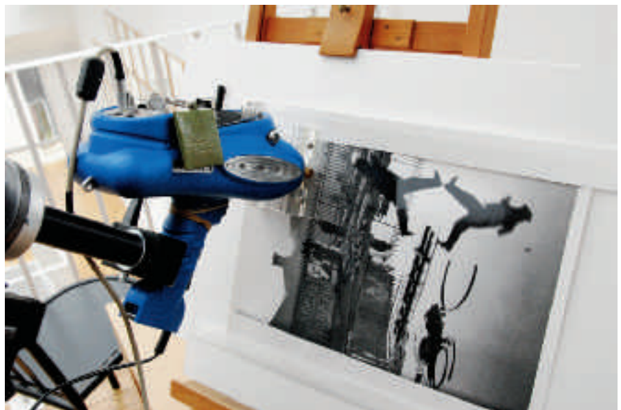
6. Quantitative XRF analysis of the Cartier-Bresson photograph, Paris. Place de l’Europe. Gare Saint Lazare. 1932 at the HCB Foundation in Paris. Photo: Dusan Stulik.
