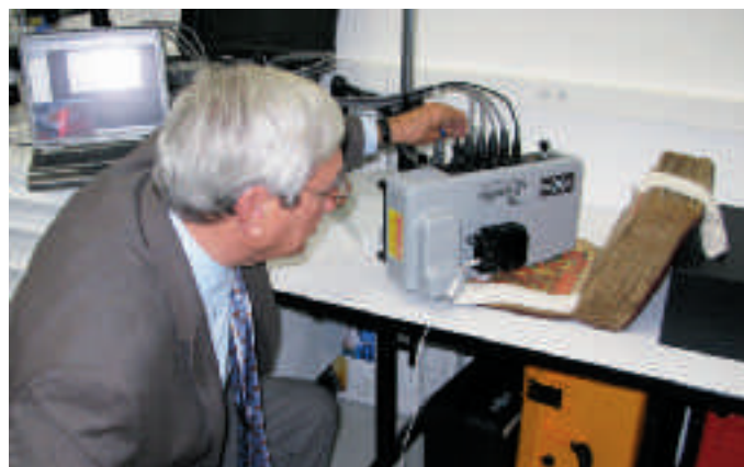
10. GCI chief scientist Giacomo Chiari uses the portable XRD/XRF to analyze pigments found in an Ethiopian gospel manuscript owned by the Getty.
