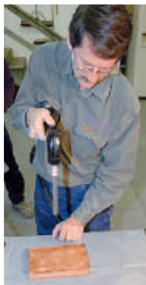
4. Randell Heath, owner of Coldsweep, Inc., cleaning a test book with dry ice misting in Mountain Green, Utah, USA. © Randy Silverman
