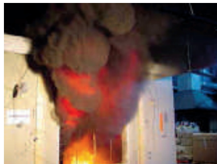
1. Two consecutive fires maximized smoke exposure to the samples; pictured here, a blazing mattress. © Alex Bwalya for NRC National Fire Laboratory
