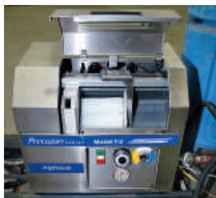
3. Block of dry ice loaded into an Alpheus Precision Series TM Model T-2 manufactured by Cold Jet, Inc. © Randy Silverman
