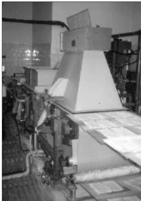
Leaf-casting system invented by the Center for Conservation Laboratory
